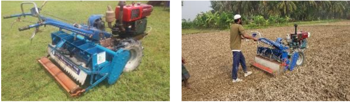
Figure 2 Pictorial view of BARI CA planter and its field operation.
