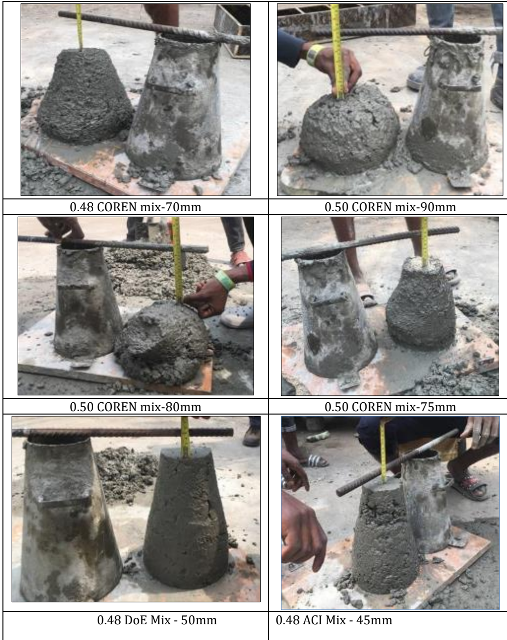
Figure 13 Slumps Testing
