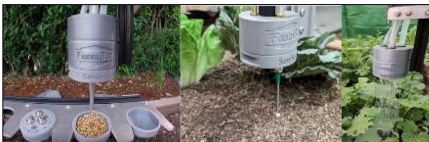
Figure 4 Farm bot precisely planting seeds and irrigation
